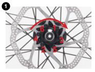
Using gloves, place the rotor onto 6-bolt hub. While applying a clockwise rotation to the rotor, tighten the bolts ¼ turn at a time following the pattern shown. Continue until the bolts are tightened to 6Nm.
