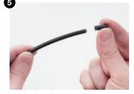
Install hooded end cap at end of housing where it meets the caliper. If there are sections of open cable, install lined end caps at those ends of cut housing.
