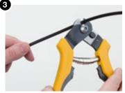
Using a sharp housing cutter cut housing to length.
