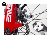
Install and crimp cable tip.
