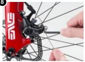
Feed cable through adjusting barrel and cable fixing plate on the caliper. Do not cut cable until caliper installation and adjustment are complete.
