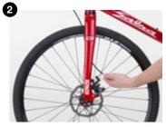
Measure the length of housing needed. Ensure housing makes smooth bends between cable stops and that handlebars can rotate completely in both directions without pulling housing taut.
