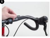
Install EZ-Bend housing into brake lever body, ensuring housing is seated fully.
