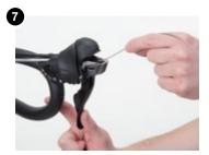
Feed cable through brake levers and housing.
