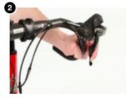
Pull brake lever until it cannot be pulled further and hold.
