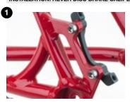
Consult the table to determine if you need an adapter for your frame or fork. If using an included Rever adapter, install and torque fixing bolts to 6–8Nm. If using an adapter from another manufacturer, install according to the manufacturer's specifications.
