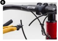
If using the included inline adjuster, cut out a 20mm section of housing. Open cut ends of housing and insert into inline adjuster. No housing end caps are needed.
