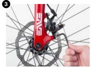
Alternating from one bolt to the other in quarter turns, tighten caliper mounting bolts to 6–8Nm. Release brake lever.
